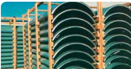
Pre-painted Column Covers, 1/4" thick Aluminum, 14 Ft. long, bump-formed to 48" Dia. With no bump lines or surface marks
