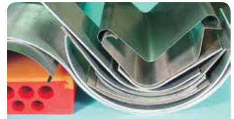
Acclaimed as the "most versatile Radius bending Tooling system in the world", SMP-1240 can bend any radius... from 3/4"(18mm) to 24"(600mm), any Gauge... up to 1/4"(6mm) S.S.
