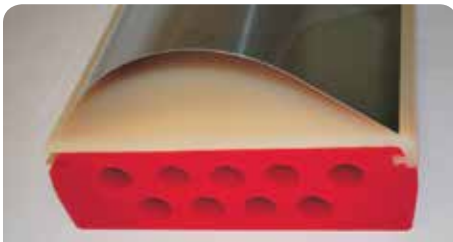
Mirror finish stainless steel trailer front corners. 5" Rad."(125mm) x 90 degrees formed in 2 hits without blend lines. Eliminated start and finishing lines from rolling.
