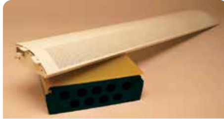
Pre-painted perforated lighting cover radius formed in one hit. Similar to Die shown below.
