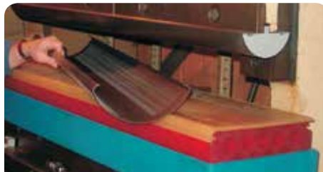
With Planers upto 30' in length we can machine steel punches of any custom shape. Custom tooling is developed on this 400 Ton Press Brake.
